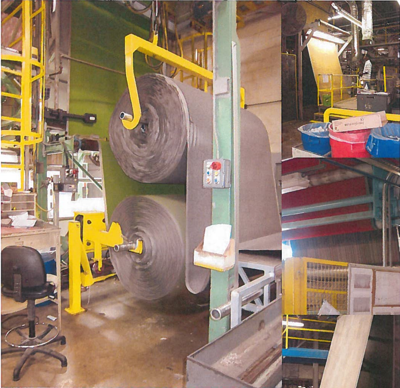
Images: Bonding the woven carpet to the carpet backing
